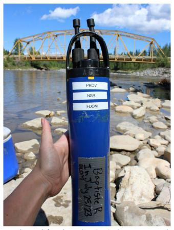
A data sonde from the Baptiste River. Sondes measure general water quality parameters, including water temperature, specific conductivity, pH, turbidity, and dissolved oxygen. Photo credit: Jillian Peterson.
