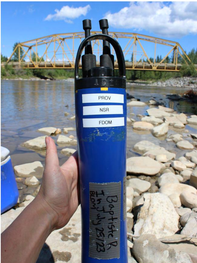
*A data sonde from the Baptiste River. Sondes measure general water quality parameters, including water temperature, specific conductivity, pH, turbidity, and dissolved oxygen.
