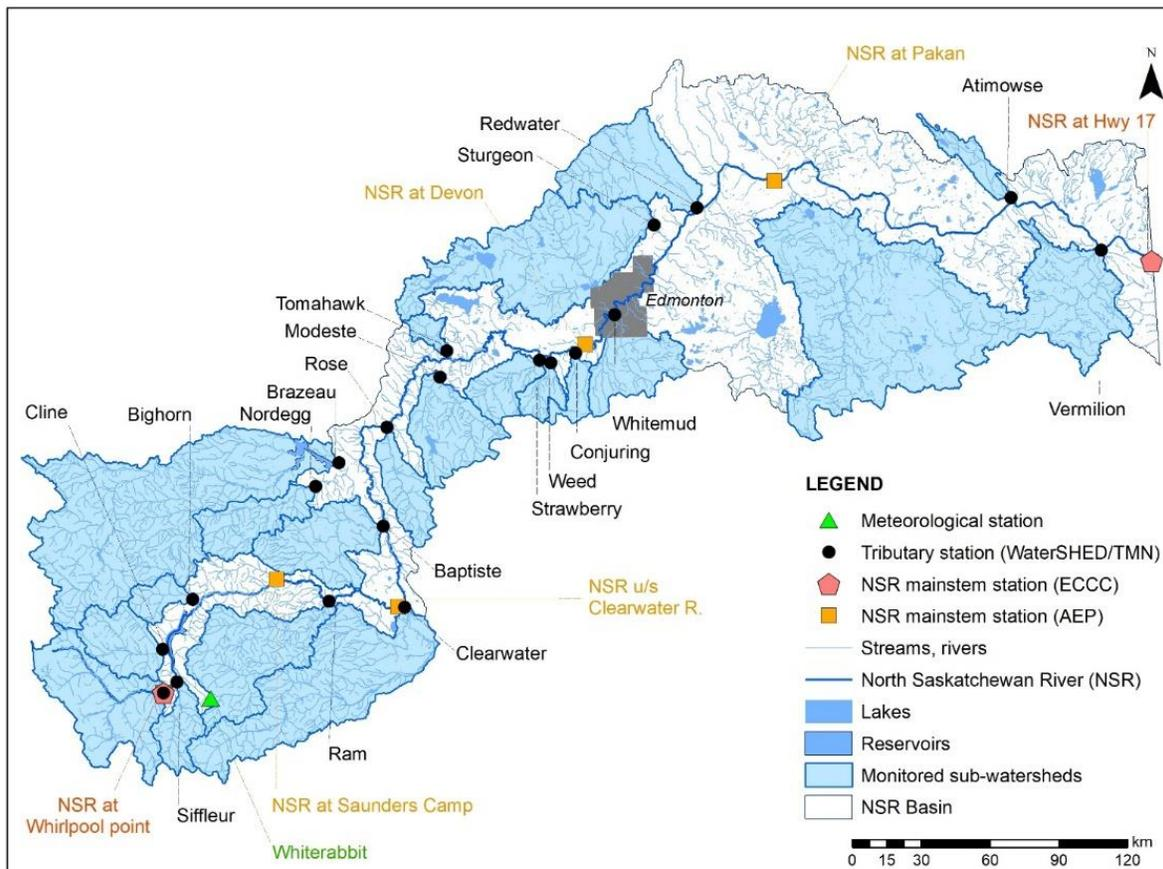
**Figure 2.** Locations of the WaterSHED monitoring stations, mainstem stations of the NSR monitored under the Government of Alberta's Long Term River Network (LTRN; Saunders, Clearwater, Devon, Pakan), and long term monitoring stations of the NSR monitored by Environment and Climate Change Canada (Whirlpool Point and Hwy 17).
