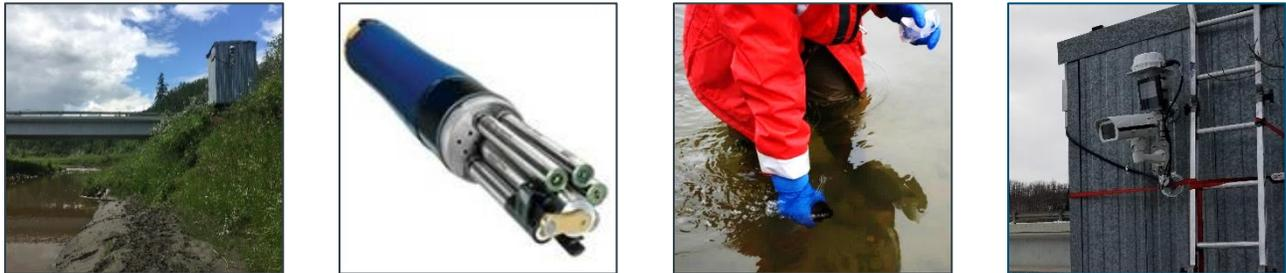
**Figure 3.** Monitoring approaches used in the WaterSHED program for monitoring river flow (left), in-river continuous water quality via data sondes (left centre), water quality grab sampling (right centre), and daily camera imagery of rivers (right).
