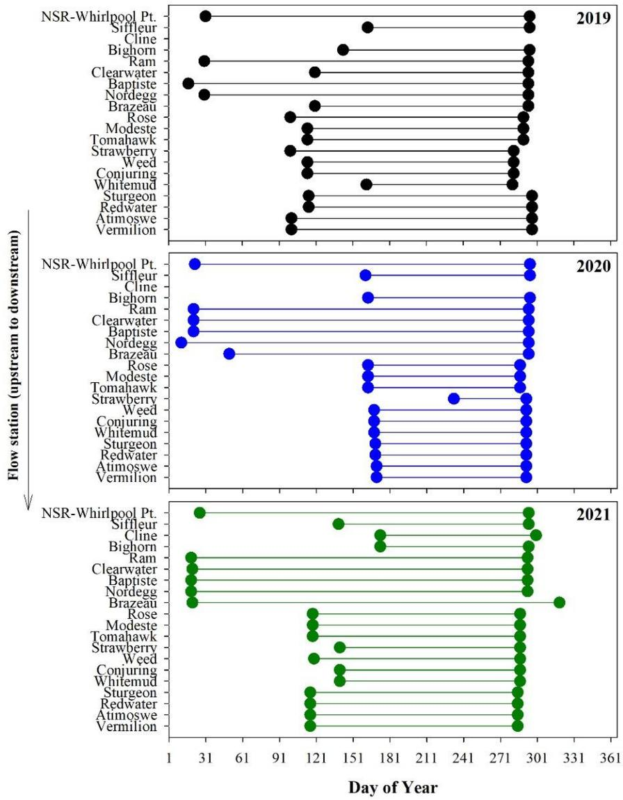
**Figure 5.** Operational history of seasonal (i.e., winter shutdown) and continuous (nearly full-year operation; removed during dynamic ice cover conditions) data sonde deployments at monitoring stations as part of the WaterSHED program; organized upstream to downstream locations.
