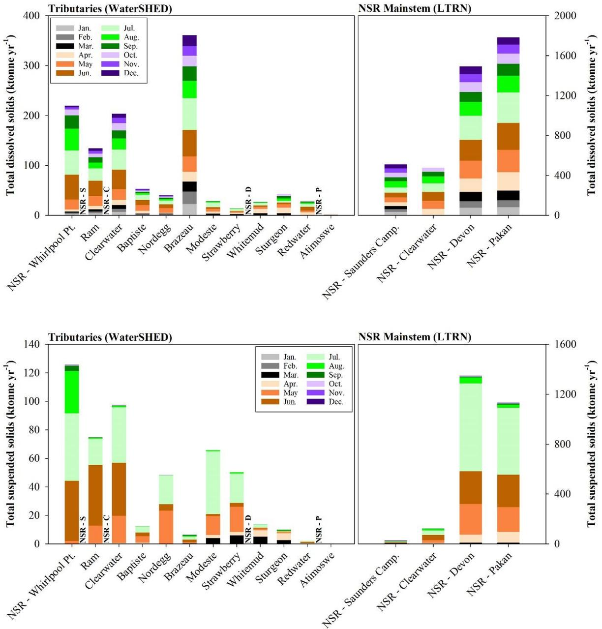
**Figure 15.** Stacked bar graphs of monthly total dissolved solids (above) and total suspended solids (below) export from selected WaterSHED monitoring stations from all samples from water years 2018-19 to 2020-21. Stations are organized upstream to downstream and relative location of LTRN stations are shown in the left panels.
