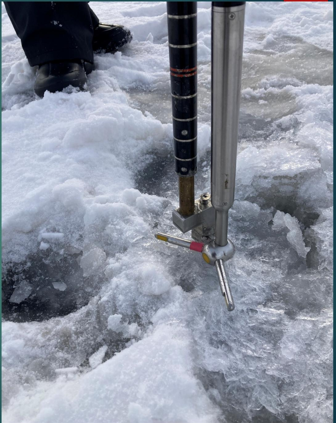
Occasionally we have to resort to old-school mechanical meters in slush conditions or in cases of equipment failure or power issues. Mechanical meters requires a beeper to count revolutions and a stopwatch to time them, both of which can be problematic in the cold. Results also have to be manually calculated.
