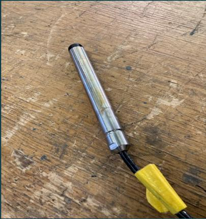
Another option is a submersible pressure transducer. These perform the same function as the bubbler, without the need to supply air through a line. They are vented to atmospheric pressure, and return a stage value to the logger.
