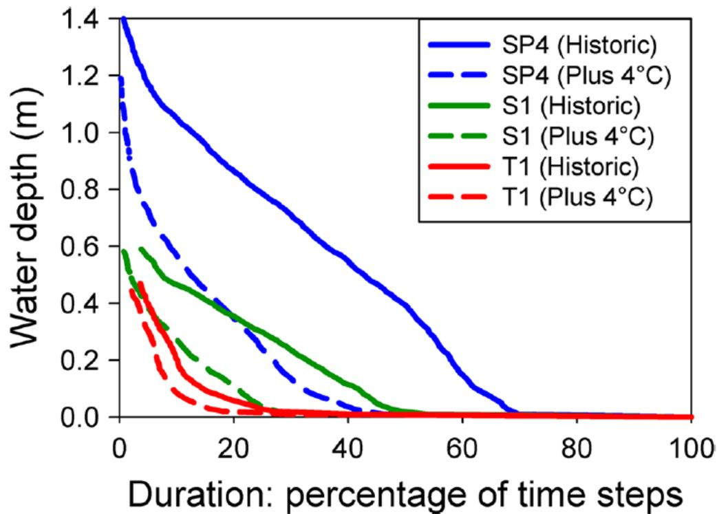
**Fig. 6** Comparison of wetland stage-duration curves from WLS for historic climate and a 4 °C climate change scenario for the Academy, South Dakota, weather station. [source: Fig. 10 in Johnson et al. (2010). Prairie wetland complexes as landscape functional units in a changing climate. *BioScience* 60:128–140]
