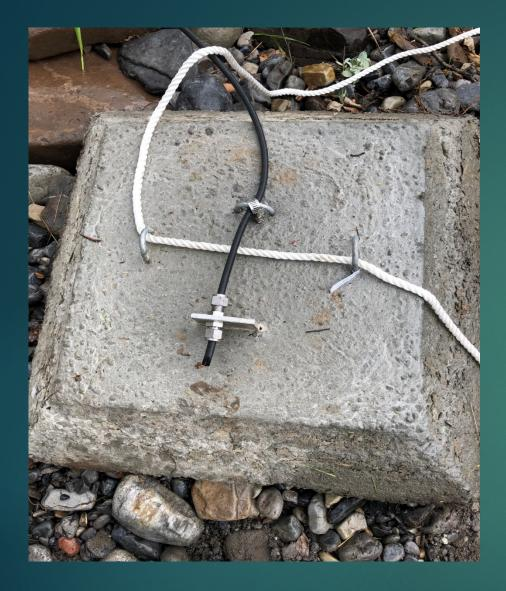
The bubbler contains a sensitive pressure transducer. Air bubbles are sent from the bubbler at a selfregulated rate of 60/minute. As the head pressure of water above the line on the streambed increases, the sensor monitors the force required to push the bubbles out the line and reflects this as water level change. It also self-adjusts to maintain that consistent bubble rate.
