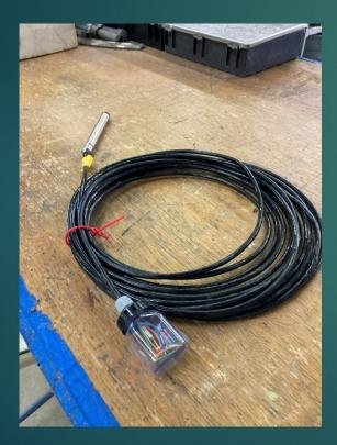
Another option is a submersible pressure transducer. These perform the same function as the bubbler, without the need to supply air through a line. They are vented to atmospheric pressure, and return a stage value to the logger. Why do we only use these is select situations?
