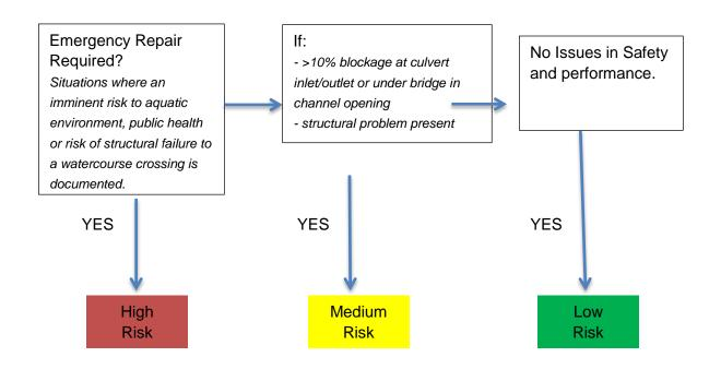
Figure 2: Safety and performance evaluation flow (McCleary et al. 2007).
