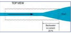
Backwater does not extend through entire culvert.
