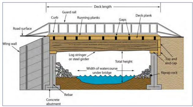
Figure 2: Bridge components evaluated for safety and performance (McClearly et al. 2006).
